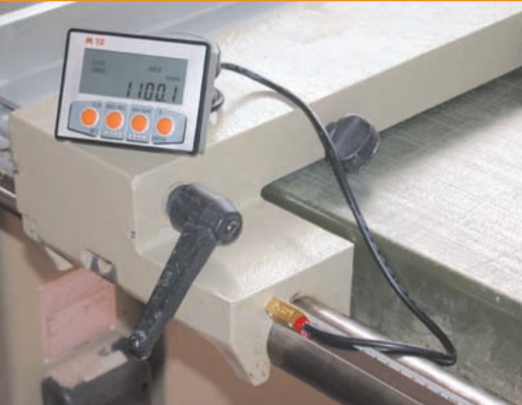
Application on mitre saws for parallel cuts
