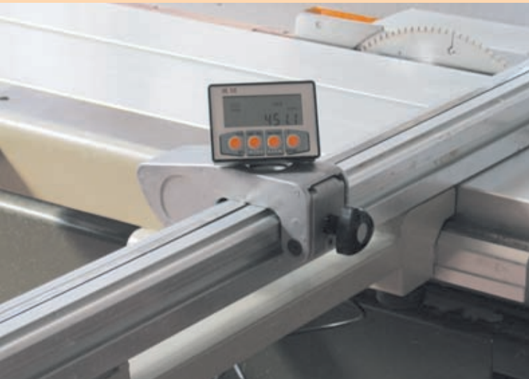
Application on panel sizing machines for squaring cuts
